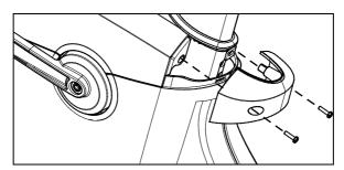
Figure 2: Rear cover removal
